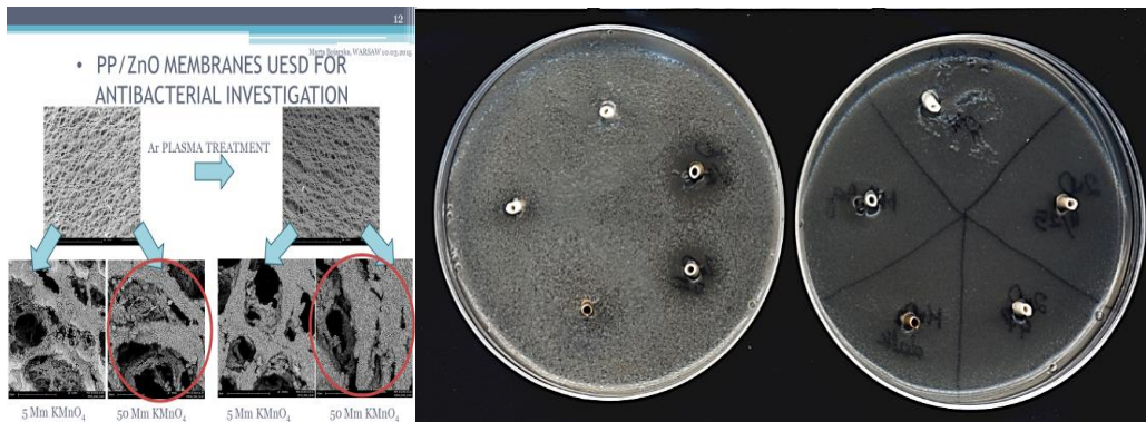
Fig. 1 A) Polypropylene membrane coated with the nanoparticle zinc oxide
